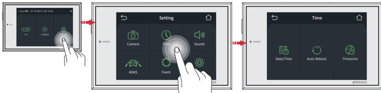
Tap on time button on the setup screen to adjust date / time, auto rebooting and time zone settings.
