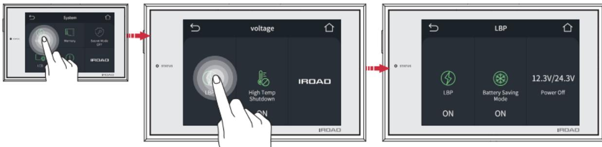
It can set up the LBP, Battery Saving Mode setting and Power off voltage.
