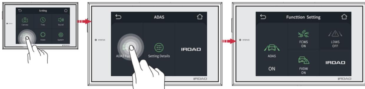
It can be controlled touch a setting button to Use or Not Use. [ADAS, FCWS, FVDW, LDWS]
