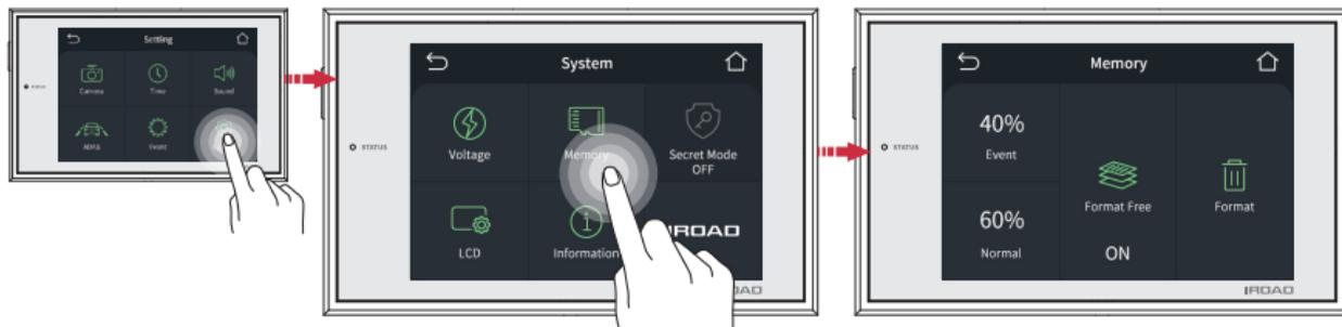
It can set up the overwrite ON / OFF, memory allocation and formatting are available.
