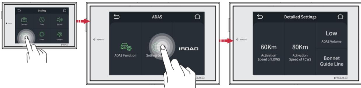
It can set up the speed for LDWS, FCWS. Thereby touch a detailed setting button as above picture.
